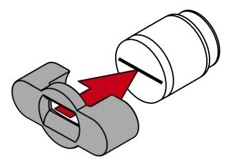
3. Align the special tool so that the logo is parallel to the recess.
