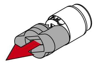
6. Push the latch inward and open the battery cover.
