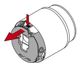
7. Remove the batteries with the special magnetic tool.
