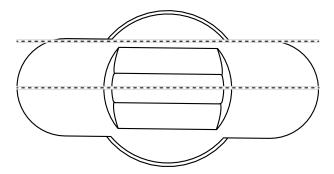
4. Hold the special tool and thumb turn cap firmly at the same time and turn them together 1-2° clockwise first and then counter-clockwise.
