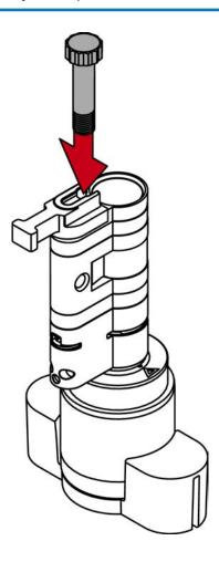
11. Reassemble the two cylinder halves.
