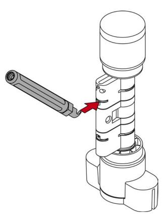
8. Lever the clamp out of the profile cylinder by moving the extractor to the centre of the cylinder.
