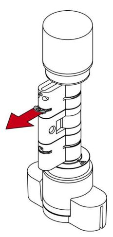
10. Disassemble the two cylinder halves.
