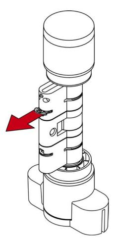
5. Disassemble the two cylinder halves.
