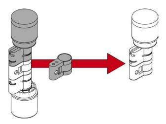
You can use a special centre piece to assemble a half cylinder from an AX comfort cylinder or a freely rotating cylinder.
