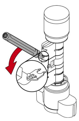
9. Pull the clamp completely out of the profile cylinder.
