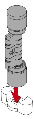
2. Attach the tip of the lifter into the clamp.
