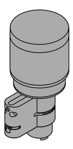
11. Place the first cylinder half on the second cylinder half.
