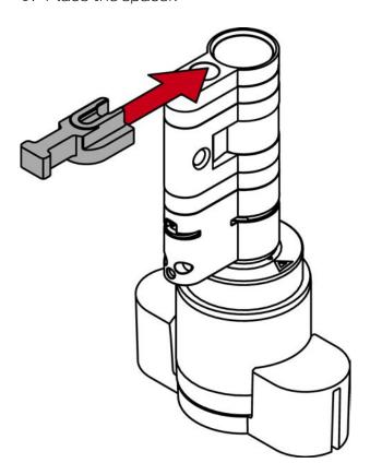
10. Screw in a suitable extension bolt with the extractor until it rests on the spacer.
