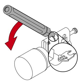
8. Pull the second clamp completely out of the profile cylinder.
