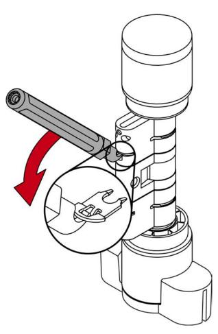
4. Pull the clamp completely out of the profile cylinder.
