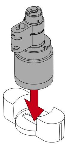
9. Place the half cylinder centre piece on the prepared cylinder half.
