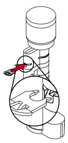
13. Insert the cylinder into the clamping block so that the profile cylinder and the thumb-turn lie flush in the recesses.
