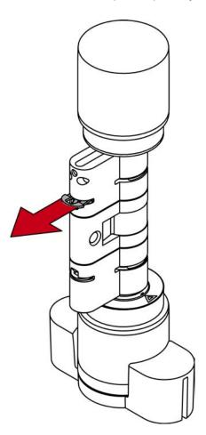
5. Disassemble the two cylinder halves.
