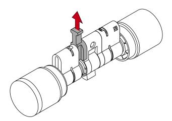
23. Push the halves together completely.
