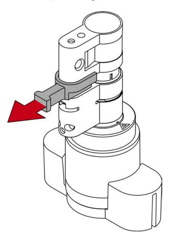
11. Push the cylinder parts together completely.
