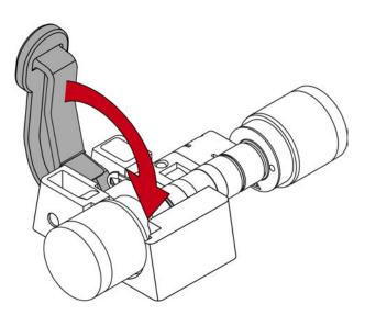
→ Freely rotating cylinder fully assembled.
