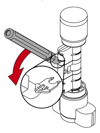
4. Pull the clamp out of the profile cylinder completely.
