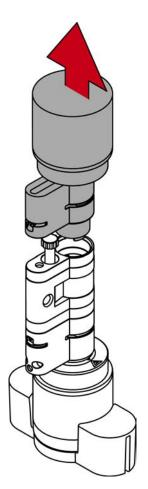
6. Unscrew the bolt with the extractor.
