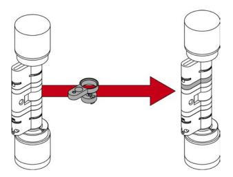
The core extension and profile extension must be the same length. You also need an extension bolt for the desired length.
