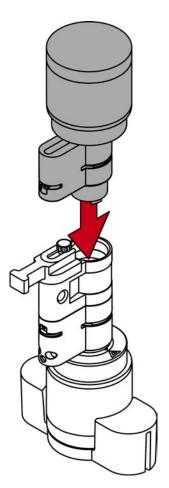
12. Refit the clip into the slot of the profile cylinder with the lug facing the fastening screw.
