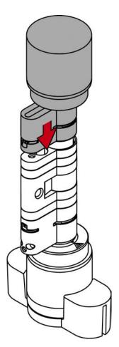
14. Place the clip back into the slot of the profile cylinder with its lug facing the fastening screw and press the clamp with your thumb so that it can no longer fall out.
