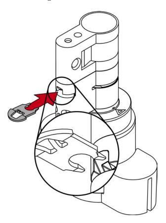
13. Insert the cylinder into the clamping block so that the profile cylinder and the thumb-turn lie flush in the recesses.
