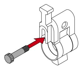
14. Place one half of the cylinder on the extension bolt.
