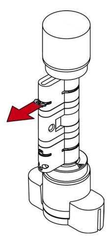
5. Disassemble the two cylinder halves.
