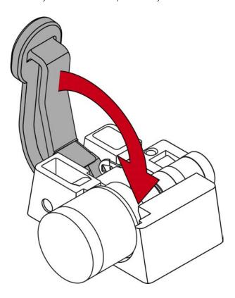
→ Half cylinder AX is fully assembled.
