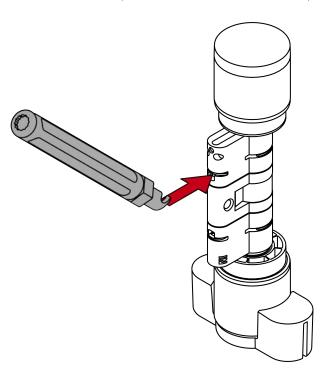
3. Lever the clamp out of the profile cylinder by positioning the lifter in the centre of the cylinder.
