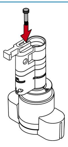
11. Reassemble the two cylinder halves.
