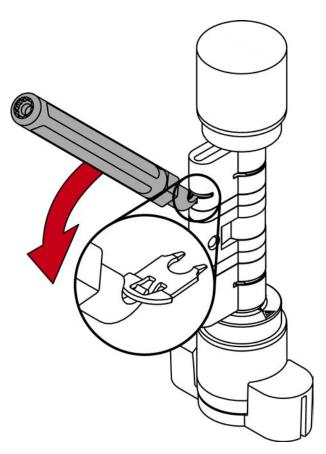
4. Pull the clamp completely out of the profile cylinder.
