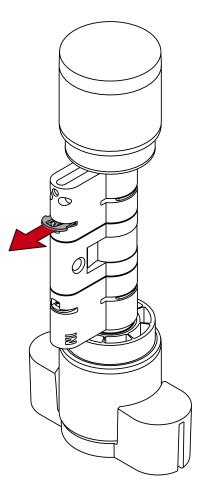
5. Disassemble the two halves of the cylinder.
