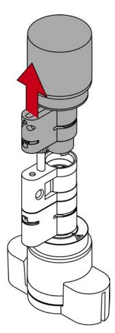
→ First cylinder half prepared with centre piece and tappet piece.
