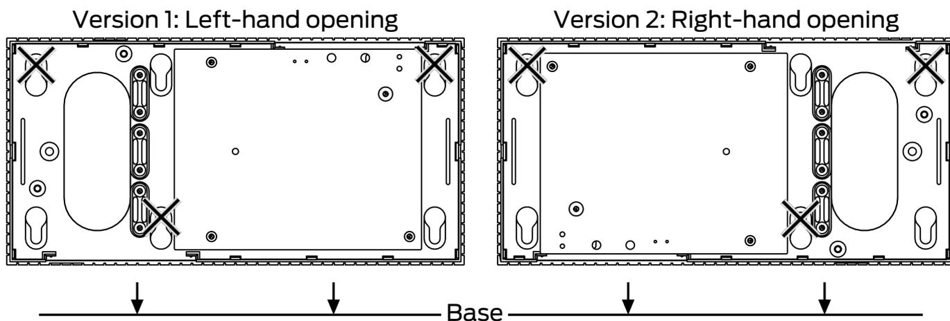
3. Drill the required holes with a suitable drill.
