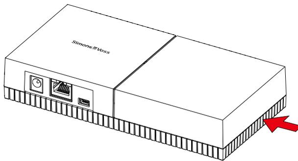
2. Check the required width of the housing opening. The height of the opening is approx. 7 mm. Each removed bar widens the opening by 4 mm.
