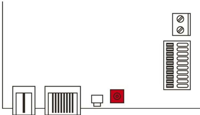
3. Connect the external antenna to the connector socket.
