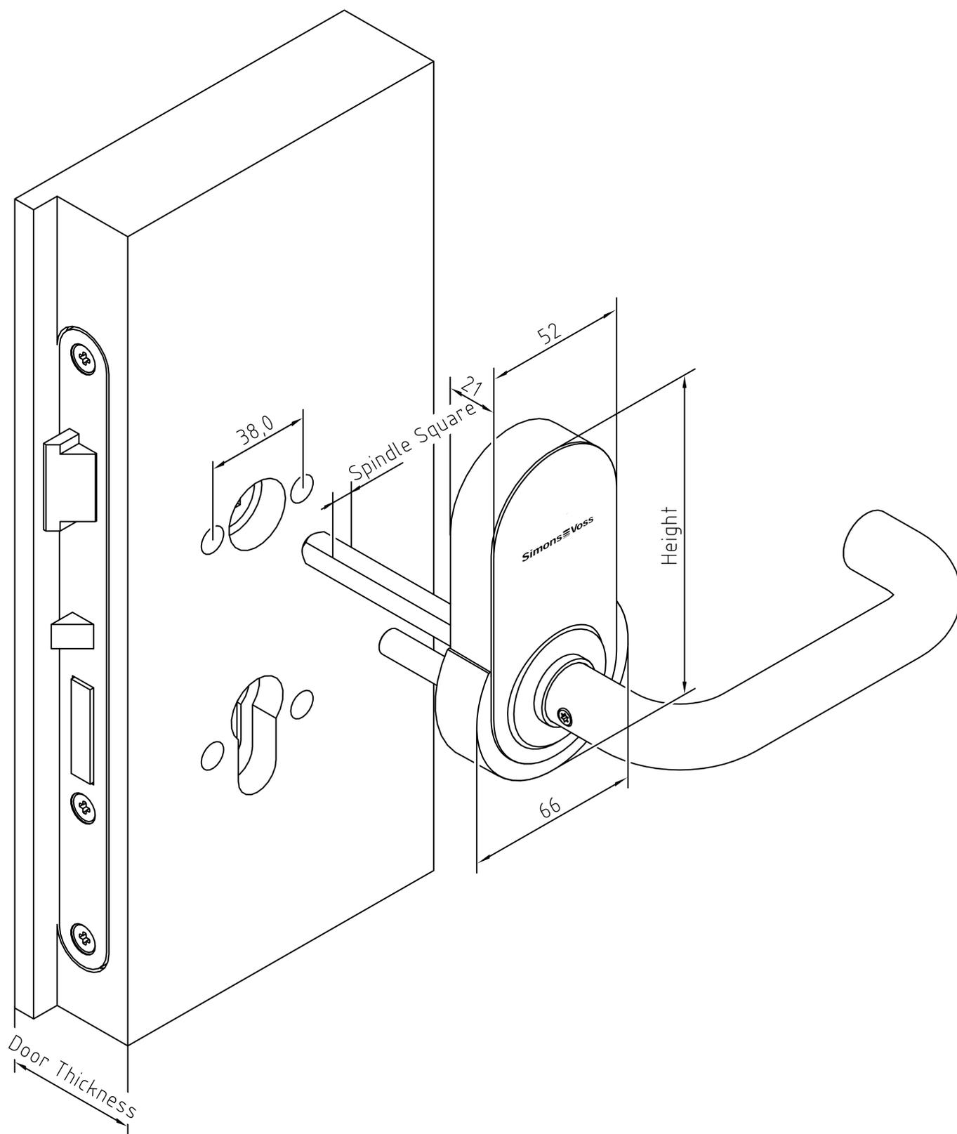
Fig. 2: Dimensioning SmartHandle AX stationary (A0)
