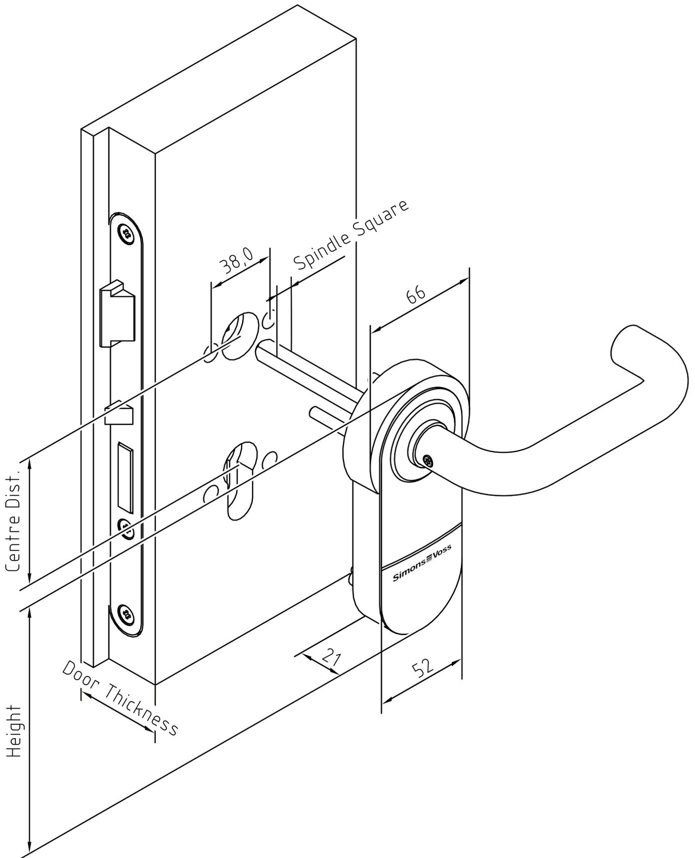
Fig. 1: Dimensioning SmartHandle AX suspended (A1, A2)
