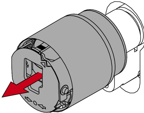
↳ Electronic thumb-turn is disassembled.
