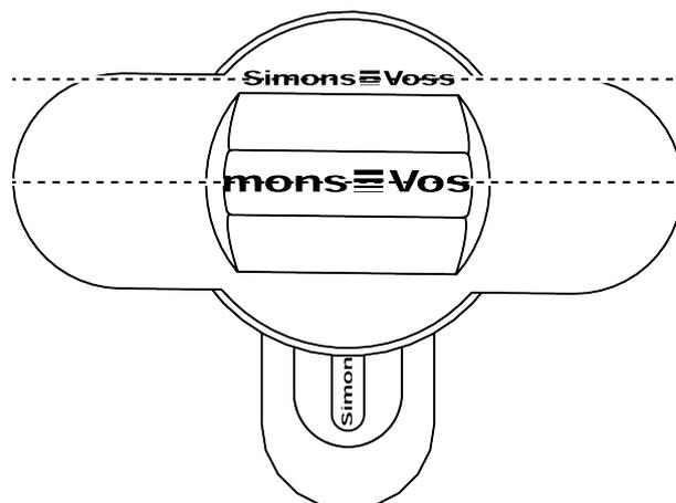
4. At the same time turn the special tool and the thumb turn counter-clockwise.
