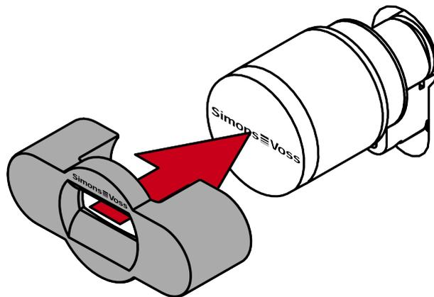
3. Align the special tool so that the logo is parallel to the recess.
