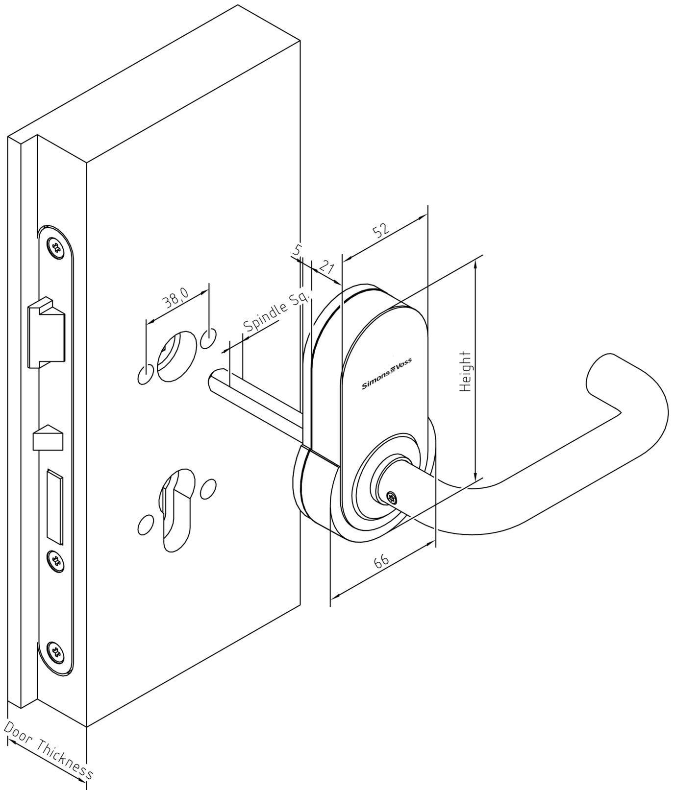
Fig. 5: Dimensioning SmartHandle AX BSL (DS)
