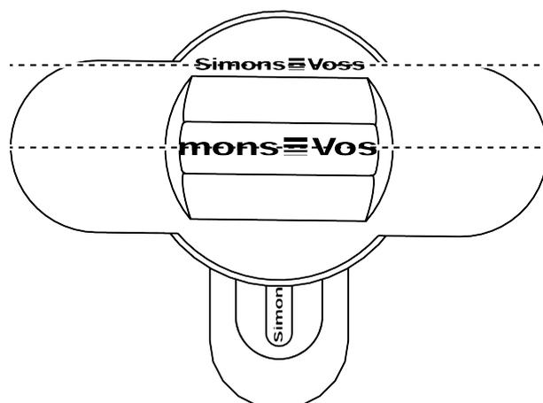
4. Hold the special tool and thumb turn cap firmly at the same time and turn them together 1-2° clockwise first and then counter-clockwise.
