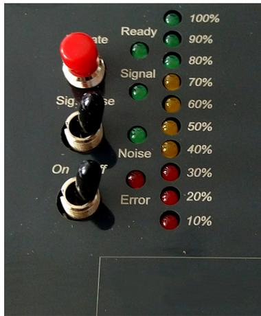
The SimonsVoss WaveNet test tool (BAMO.EU) can be used to take stock of the situation during measurement. The object in which the project is to be implemented should no longer be changed after the measurement. Therefore, measurement in an unfinished building or in a bodyshell is not recommended. The BAMO provides three values with two measurements:
