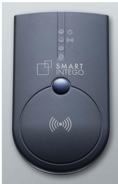
The SI.SmartCD is a local USB programming device and is used by the SmartIntego tool:
