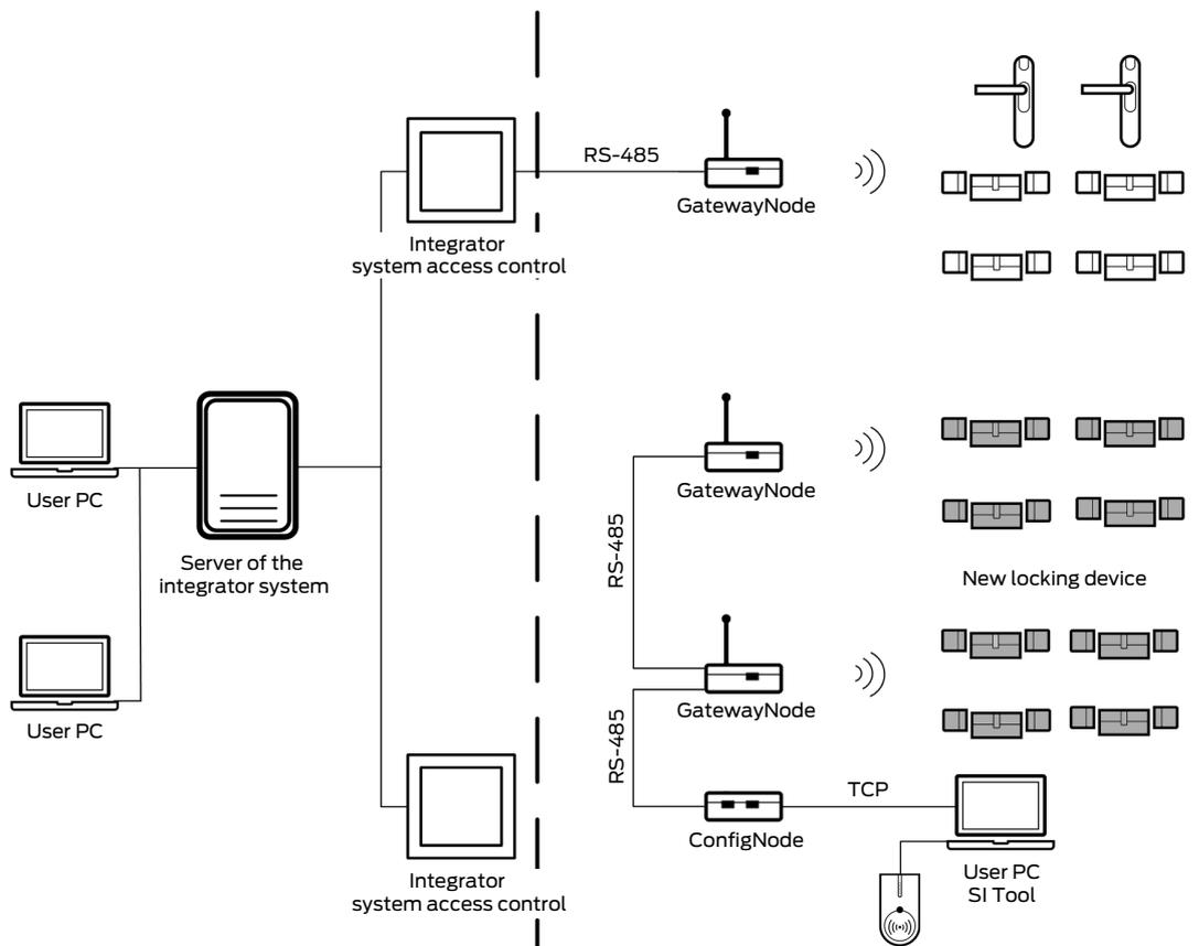
In this example, the grey locking devices are no longer connected to the integrator system and are offline.
