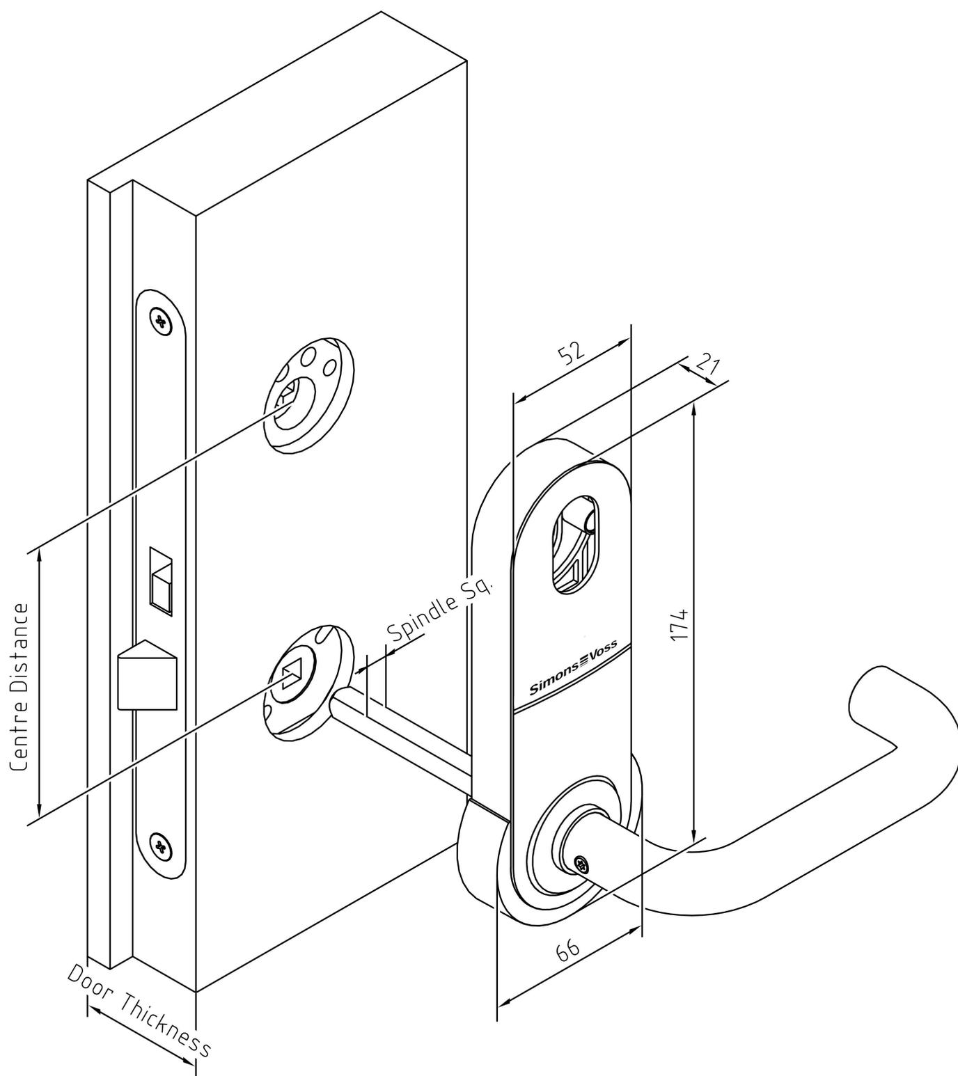
Fig. 3: Dimensioning SmartHandle AX Scandinavian Oval (E0, E1)
