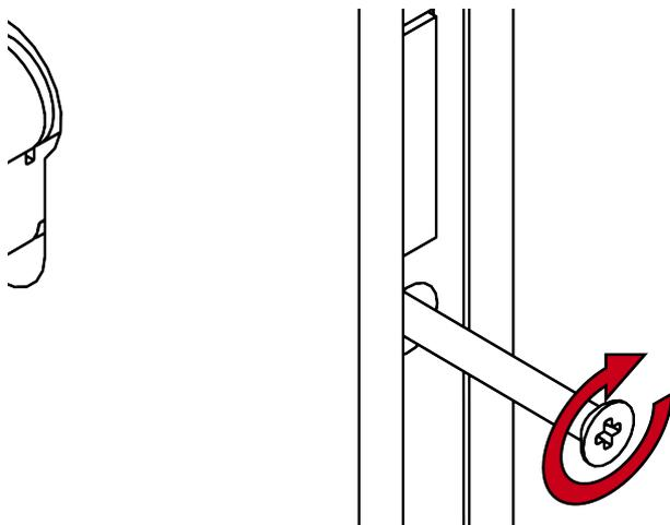
↳ Locking cylinder AX is fixed in the lock.
