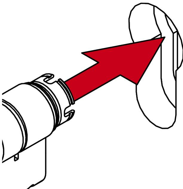
↳ You have positioned the AX locking cylinder in the lock.
